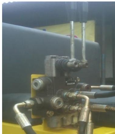
Gambar 2.7. *Control valves tipe multiple*
