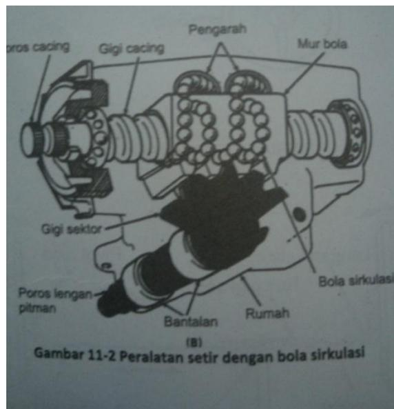
Gambar 2.3. *Recirculating ball gear*.<sup>14</sup>
