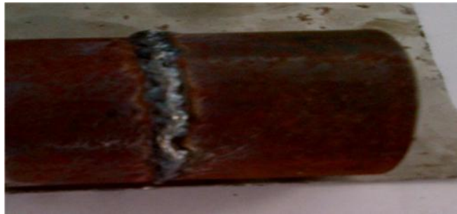
Gambar 4.15. hasil Pengelasan pipa job 6
