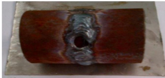
Gambar 4.10. hasil Pengelasan pipa job 1
