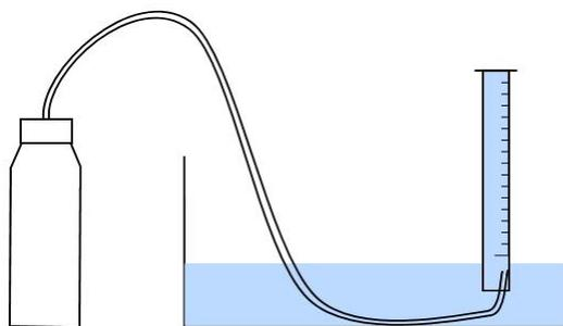
Gambar 3. 4. Metode Pengukuran Volume Gas HHO
