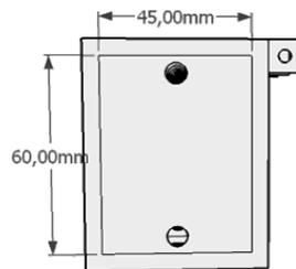
Gambar 3. 7. Layout Elektroda Generator Elektrolisis Dry Cell
