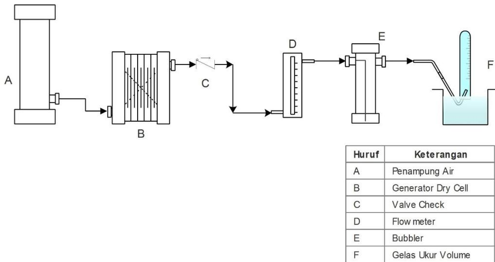
Gambar 3. 10. Proses Kerja Generator elektrolisis Tipe Dry Cell
