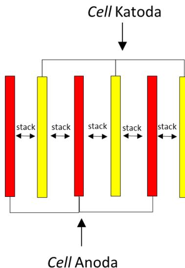
Gambar 3. 6. Konfigurasi Cell Generator Elektrolisis Dry Cell
