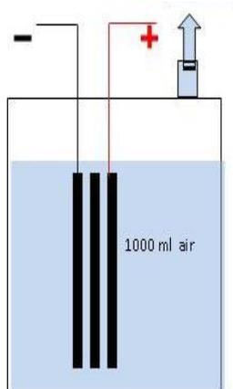
Gambar 2. 11. Tipe Generator elektrolisis HHO Wet Cell
