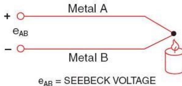
Gambar 2. 9. Cara Kerja Termokopel Tipe-K
