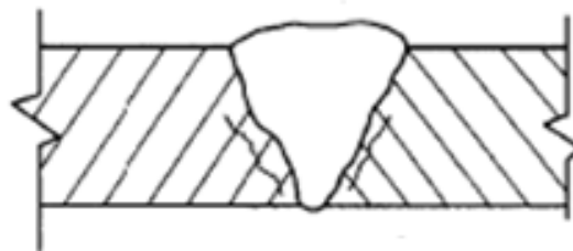
Gambar 2.27 Cacat Las Internal Underbead Crack 70
