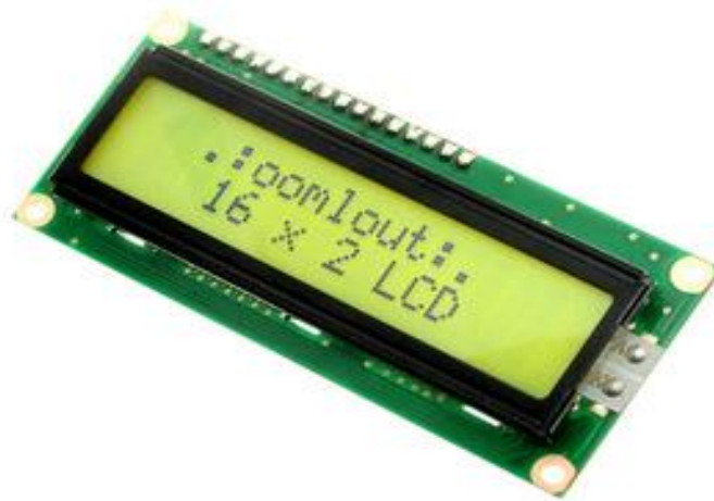
Gambar 2.14. LCD (Liquid Cristal Display)
