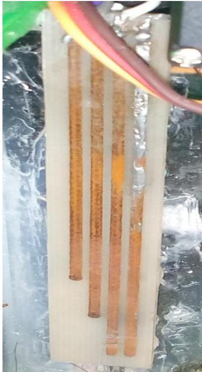
Gambar 2. 3 Water Level Sensor
