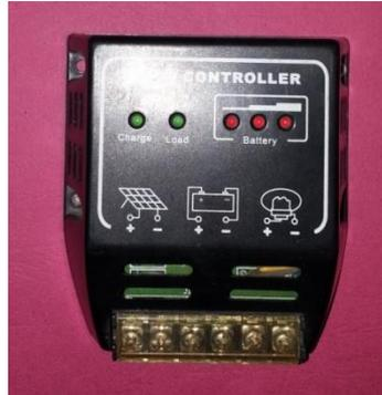
**Gambar 2.13. Charge Controller PWM (Pulse Width Modulation)**
