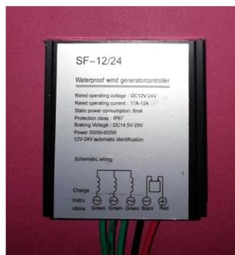
**Gambar 2.14. Generator Wind Controller**
