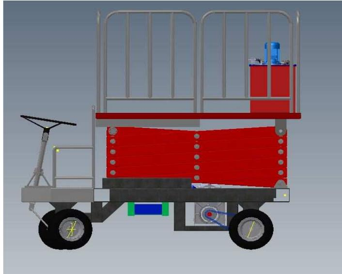
Gambar 3.2 Mesin *Scissor Lift*
