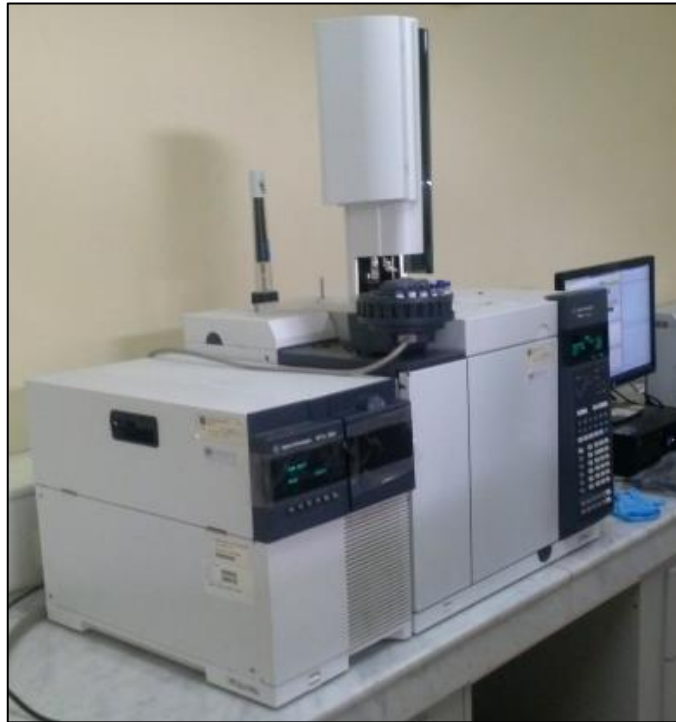
Gambar 2.6. Gas Chromatography-Mass Spectrometry (GC-MS) Agilent Technologies 5977A MSD - DB WAX column (NIST mass spectral database).
