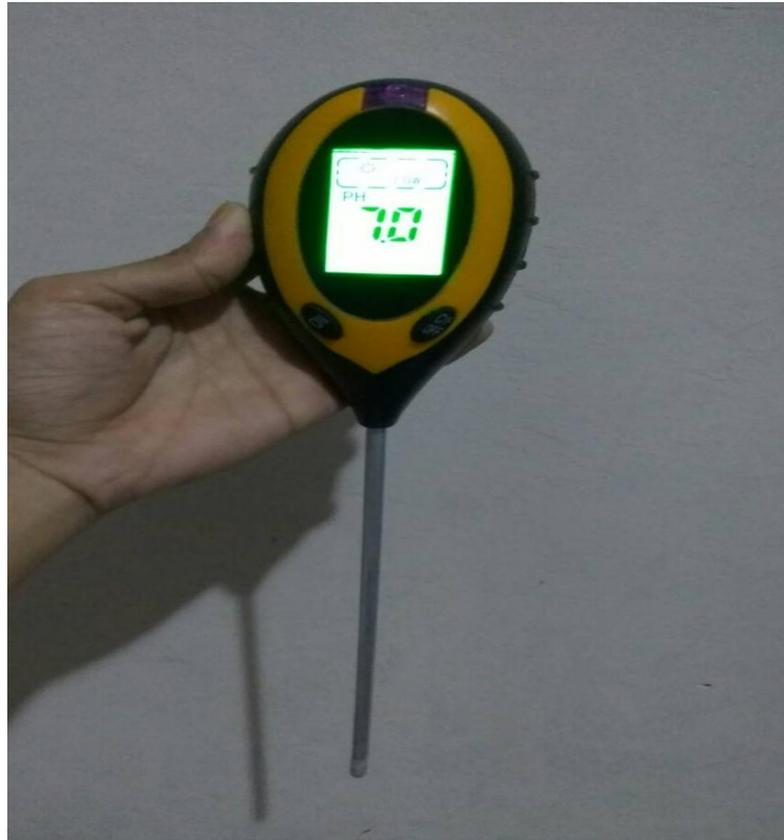
Gambar 9. Alat Soil Tester
