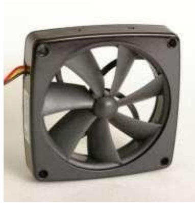
Gambar 3.12 exhaust / kipas pendingin CPU
