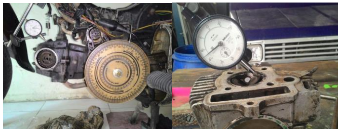
Gambar 3.14 Pengukuran Valve Timing Rocker Arm & Lift Valve
