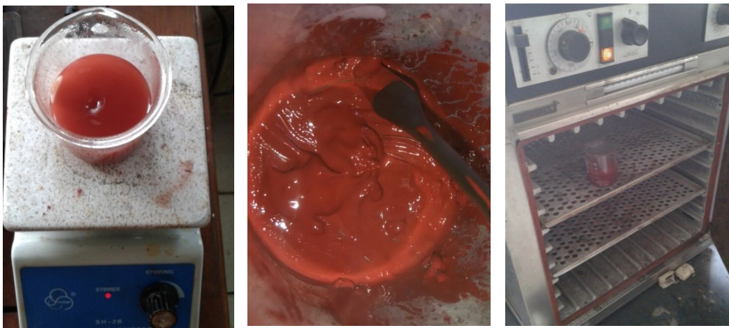
Gambar 4.1. Preparasi material \text{BaFe}_{12-2x}(\text{ZnCo})_x\text{Ti}_x\text{O}_{19}
