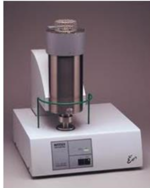
Gambar 2.9 Alat uji Analisis Termal Diferensial ( Differential Thermal Analysis, DTA )
