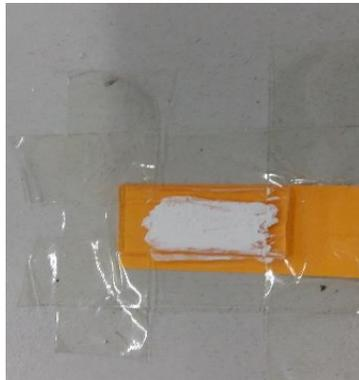
**Gambar 3.5** Skema Area Deposisi Pasta  $\text{TiO}_2$
