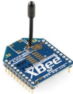
Gambar 2.11. Xbee 2mW Wire Antenna - Series 2 (sumber: http://examples.digi.com )
