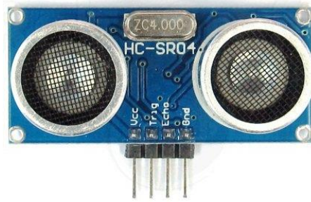
Gambar 2.3. Sensor Ultrasonik (sumber: https://electrosome.com )
