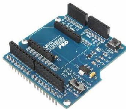
Gambar 2.12. Bluetooth Bee V03 Shield (sumber: http://sensorembedded.com )
