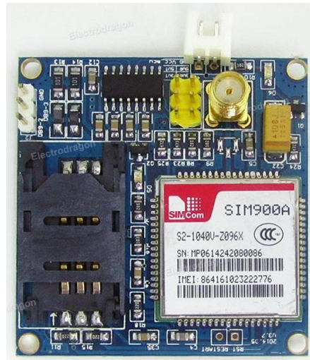
Gambar 2.13. GSM SIM900A (sumber: http://electrodragon.com )
