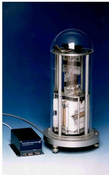
Gambar 8. *Fluxgate* magnetometer
