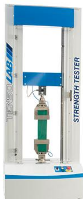
Gambar 3.1 Tensolab 5000 Strength Tester
