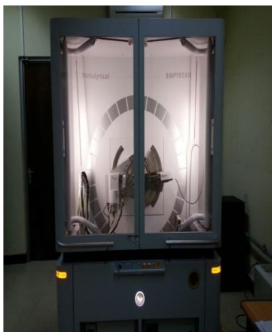
Gambar 12. Alat uji X-Ray Diffraction (XRD) PANalytical JEOL JSM-6510LA.
