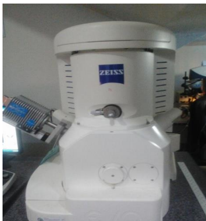
Gambar 11. Alat uji Scanning Electron Microscopy (SEM) EVO MA10.
