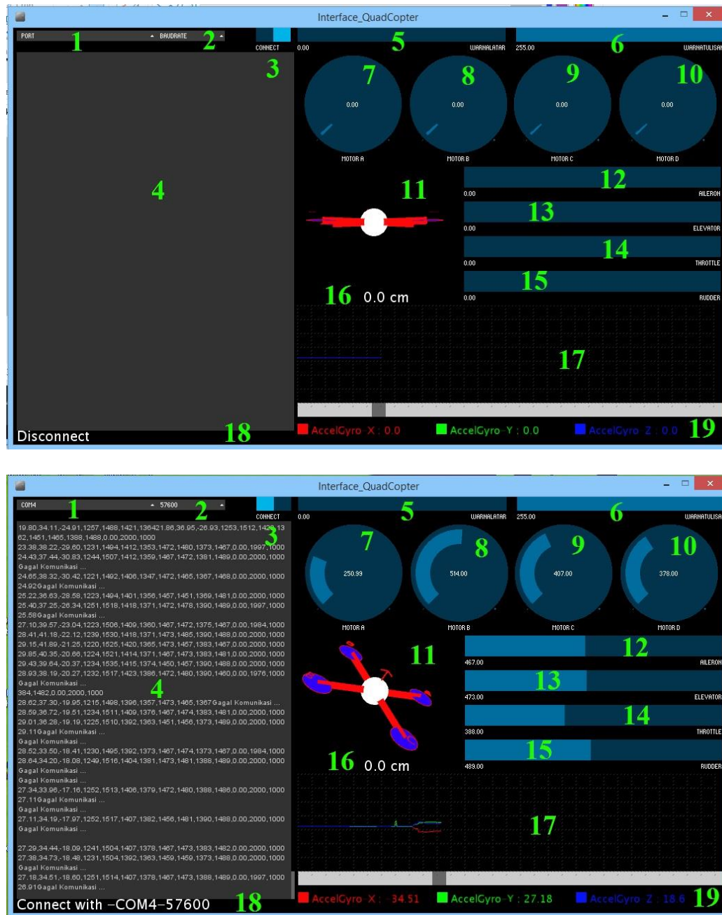
Gambar 3.5. Desain Program HMI Quadcopter Robot
