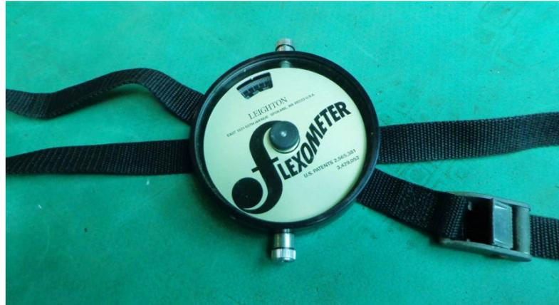
Gambar 3.2 Alat pengukur *flexibility* (*Flexometer*)
