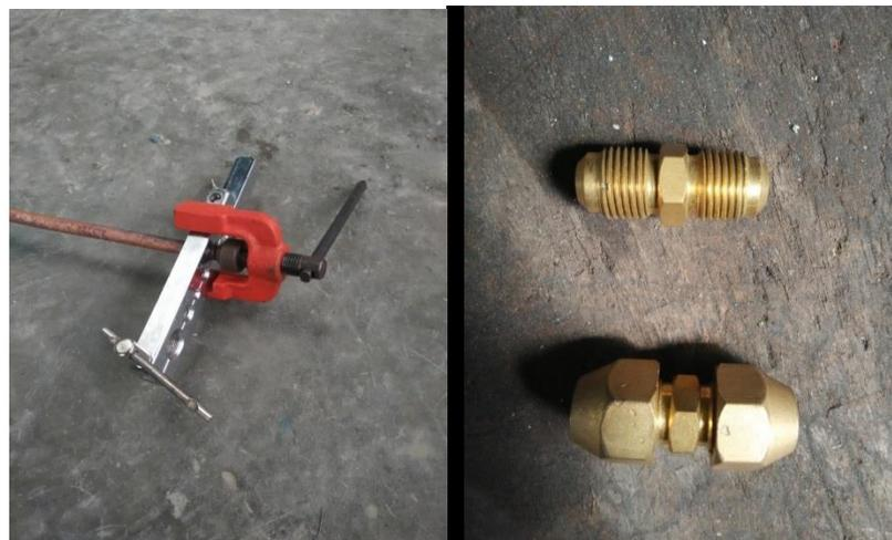
**Gambar 3.1. Flare Fitting Dan Flare Nut(Double Nipple)**
