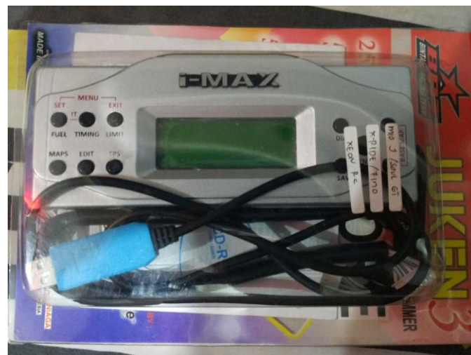
Gambar 3.3 Remote Programmable ECU BRT Juken 3
