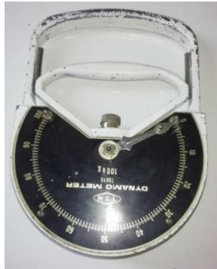
*Gambar 10: Grip Strenght Dynamometer
