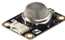
Gambar 2.1 Sensor Gas MQ2
