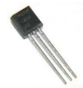
Gambar 2.2 Sensor Suhu LM35
