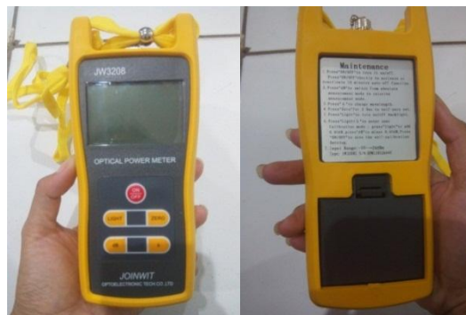
Gambar 3.5 OPM ( Optical Power Meter )
