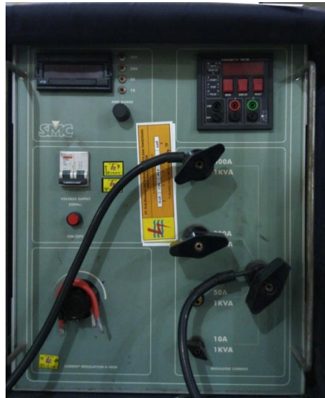
Gambar 3.1 Primery Injection Test Set LET 400 RD
