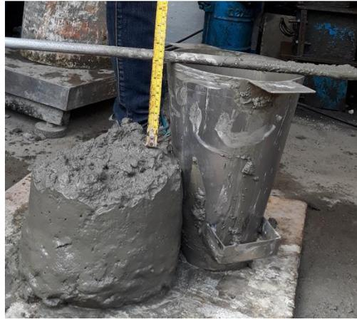
**Gambar 4.2 Slump Beton Normal**
