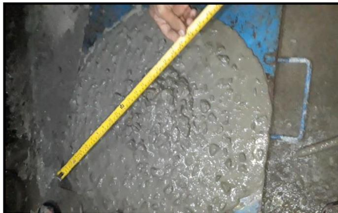
**Gambar 4.1 Slump Flow Beton Speedcrete**
