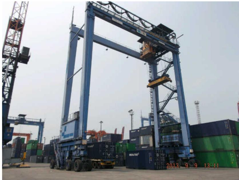
Gambar 2.1, Rubber Tyre Gantry
