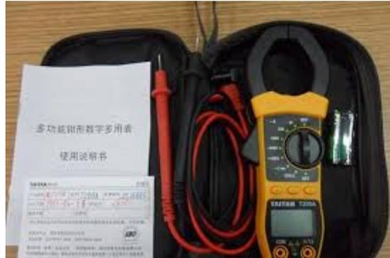
Gambar 2.29, Clip-On Ammeter (Clampmeter)
