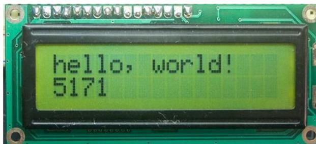
Gambar 2.9 *Liquid Crystal Display* 2 X 16
