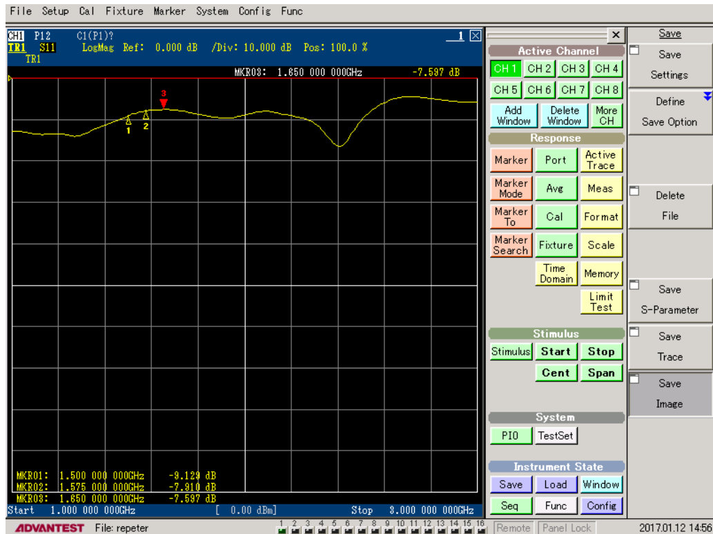
Gambar 4.21 Hasil Pengukuran S_{22} ( Output Return Loss )
