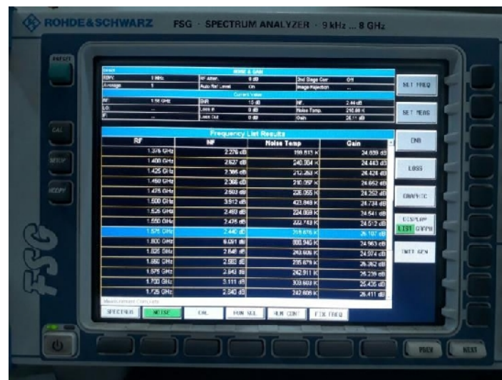
Gambar 4.19 Hasil Pengukuran Noise Figure
