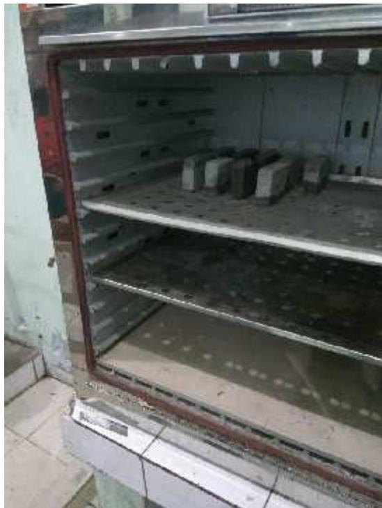
Gambar 9. Benda uji kering oven 24 jam
