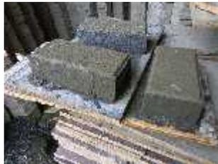
**Gambar 1.4 *Paving block* Hasil Pencetakan**
