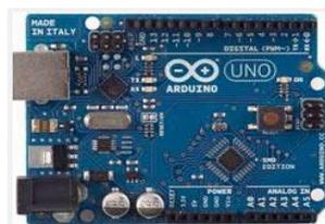
Gambar 4. Board Arduino Uno
