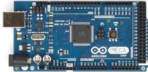
Gambar 2.3 Arduino Mega
