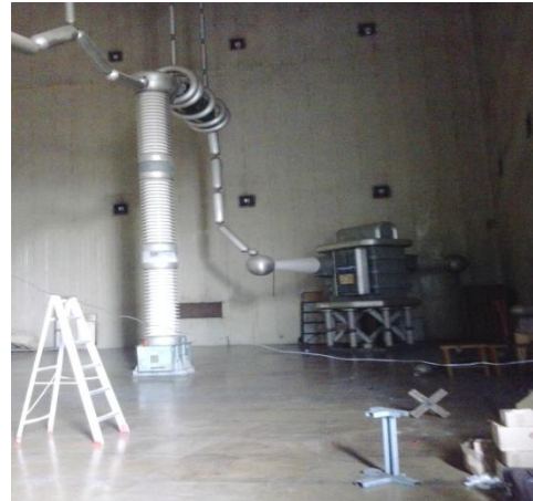
Gambar2.3 Tes set Partial Discharge di laboratorium Gdg.4
