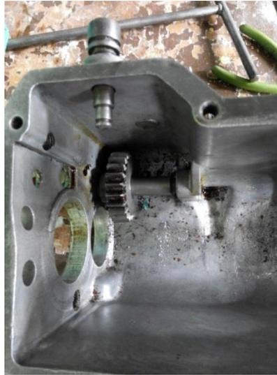
Gambar 2.4 *Reverse Idle Gear and Shaft*
