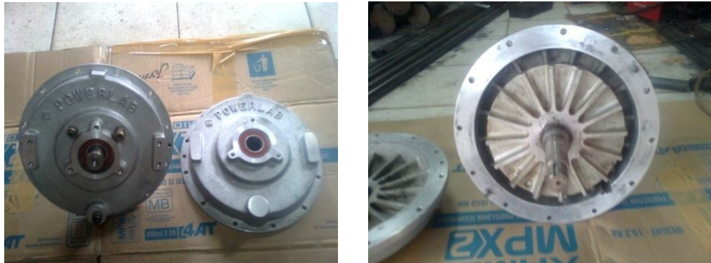
Gambar 3.8 Membongkar Housing Water Brake Dynamometer
