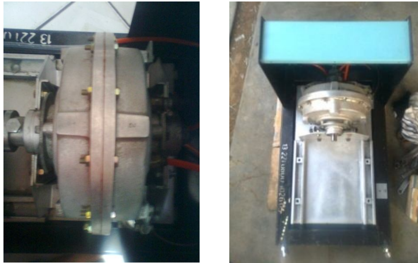
Gambar 3.10 Pemasangan Housing Water Brake Dynamometer
