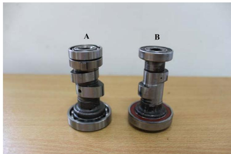
Gambar 3.5 ( A ) Noken as / *Camshaft* Standar ( B ) Noken as / *Camshaft* yang Sudah Diubah
