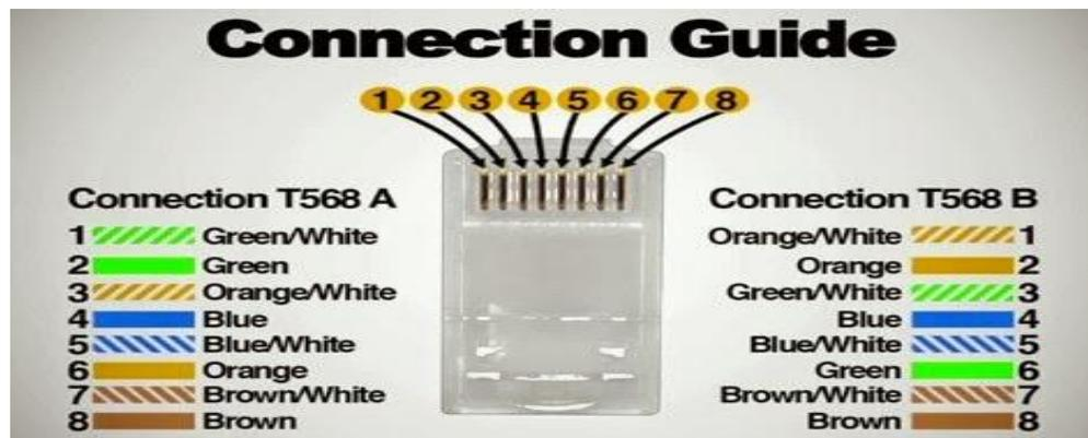
Gambar 2. 6 Straight Through Cable dan Cross Over Cable
