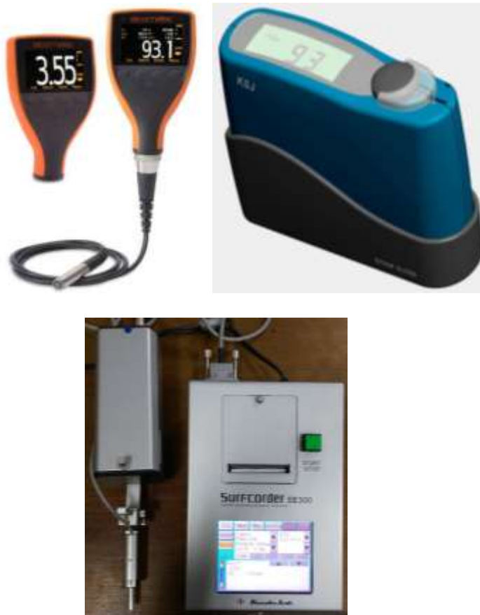
Gambar 4.11 thickness gauge, gloss meter dan roughness test.
