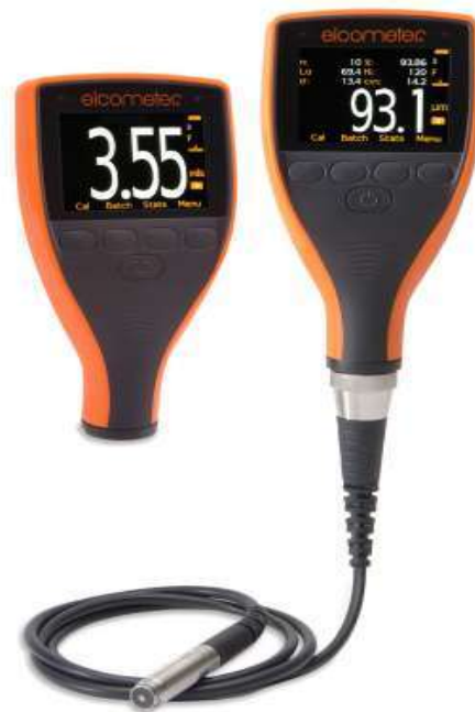
Gambar 2.18 alat ukur ketebalan cat ( Elcometer )
