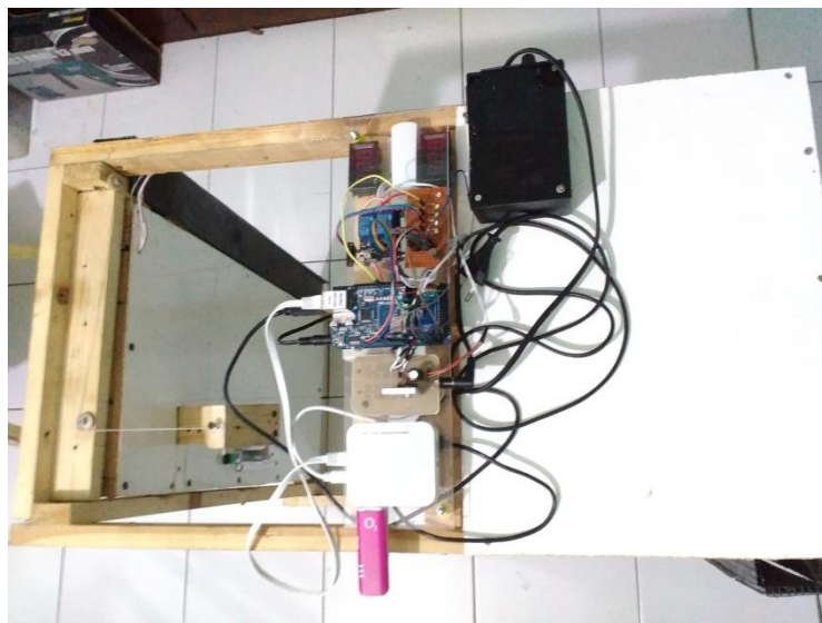
Gambar 4.5. Box Panel Kontrol
