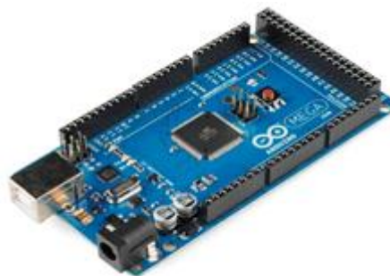
Gambar 2.4. Arduino Mega 2560 (Sumber : Kadir, 2015)
