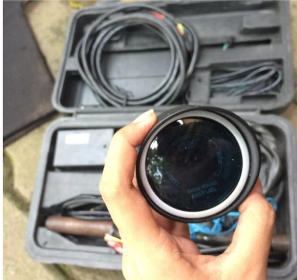
**Gambar 3.2** *Wide Band Air Fuel Ratio Meter*
