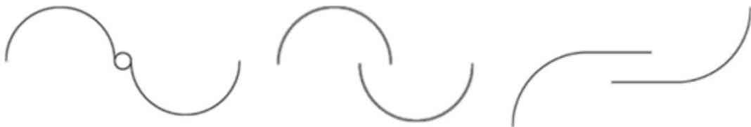
Gambar 2.3 Turbin Savonius Tipe U, Tipe S, Tipe L
