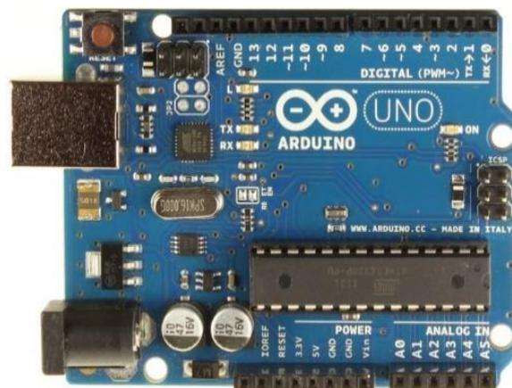
**Gambar 2.14. Papan Arduino Uno**
