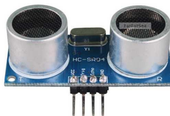
Gambar 2. 4 Modul Sensor Ultrasonik HC-SR04 Sumber : (Indoware, 2013, hal. 2)
