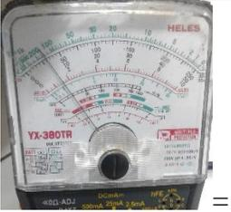
= 1.2VDC<br>Perhitungan = 1.25VDC<br>$\frac{63,75}{255} \times \frac{x}{5} = 1.25VDC$ |
