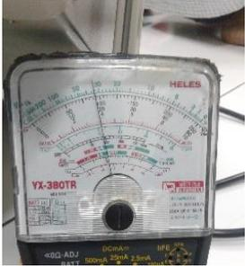
= 3.75VDC<br>Perhitungan = 3.75VDC<br>$\frac{191,25}{255} \times \frac{5}{1} = 3,75VDC$ |
