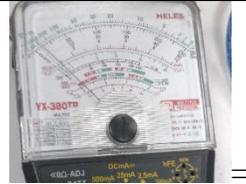
=1.5VDC<br>Perhitungan = 1.5VDC<br>$\frac{191,2}{255} \times \frac{x}{2} = 1.5VDC$ |
