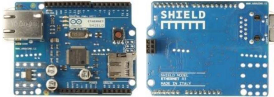
Gambar 2.14. Arduino *Ethernet Shield Wiznet W5100*
