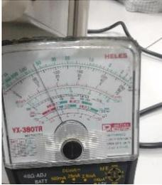
= 2.5VDC<br>Perhitungan = 2.5VDC<br>$\frac{127,5}{255} \times \frac{5}{1} = 2,5VDC$      |
