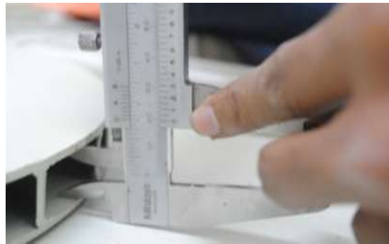
Gambar 4.6. Lebar Sudu Turbin Cross Flow
