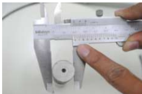
Gambar 4.4. Poros Diamater Turbin Cross Flow
