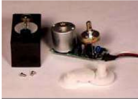
Gambar 2.17 Sistem Mekanik Motor Servo
